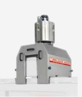
Exhaust unit with microfilter An exhaust unit can be placed over the spray hood to suck up excessive oil mist that is created during spraying. Centrifugal force will separate the oil from the air. The removed oil is discharged via a hose and collected in a container. Clean air is blown out through the filter.
