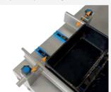
Collecting trays Sliding collecting trays are attached to each side of the conveyor belt.
