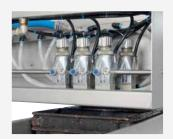
B Customized solutions: Different positions of the spray guns are possible (e.g. 6 in a row, 2 rows of 3)
