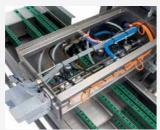
C Automatical conveyor Trays, etc. are transported by 2 chains. The motor is thermally protected.
